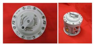
RJB11S1500 Explosion-proof isolator and selector switches up to 4p 32A 11kW AC3. Feature padlockable handle, cable entries in the bottom side or topbottom. Mounting base with 4 fixing points. External equipotential bonding connection facility for 4-6 mm<sup>2</sup> wire. Models normally available ex-stock:
