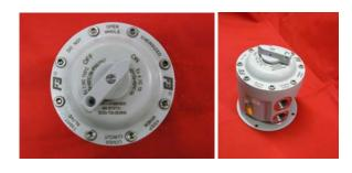
RJB11S1500 isolator and selector switches up to 4p 32A 11kW AC3. Feature padlockable handle, cable entries in the bottom side or top-bottom. Mounting base with 4 fixing points. External equipotential bonding connection facility for 4-6 mm<sup>2</sup> wire.
