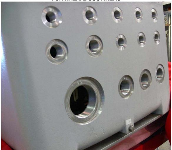
Threaded entry holes are always marked with thread type and size. Metric (parallel) threaded entry holes are always provided with a flat spot-face to ensure accurate sealing and the highest IP protection level of the entry device.
