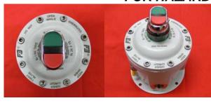
RJB11S2008 Key Switch and RJB11S2009, RJB11S2010 Selector Switches. Available in a variety of configurations: 0-1, 1-2, 1-0-2, 1-2-3, AUTO-MAN, FWD-OFF-REV etc. Up to 2 separate contacts available in each position. Choice of silver 690Vac or gold quadconnect low voltage contacts.
